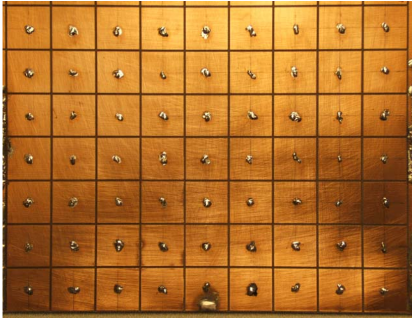
Fig. 3.13 Fabricated EBG surface using FR4 board with length 18 cm, width 18 cm and thickness
