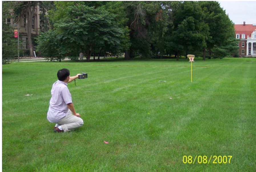
Fig. 4.10 The way we field test the reading range
